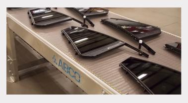
To ensure an accurate post-mold cool down, ABCO strategically positioned and bolted Delrin® support posts with PVC caps on the face of the conveyor material. The support posts allow the glass to cool properly without having to rest the glass directly on the conveyor belt.
